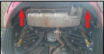
2. The middle pipe needs to be shortened – cut off 25cm measured from the flanche.
